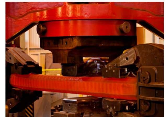
State-of-the-art facility with 4,500 ton forging press and lean manufacturing environment
