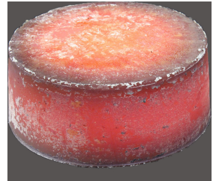
AD730® as forged disc for gas turbine
