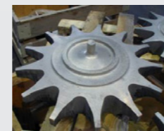
Turbine impeller U720 (85 kg – 187 lbs)
