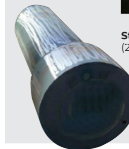
Open die forging Superalloy (3,365 kg – 7,418 lbs)
