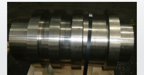
Steam Turbine Rotor Shaft – Superalloy (2,020 kg – 4,453 lbs)
