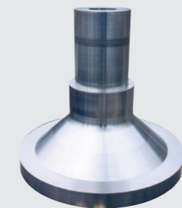
Turbine aft shaft – IN706 (9,000 kg – 19,841 lbs)
